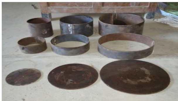
Figure 3. Model footing and model skirts used for study
